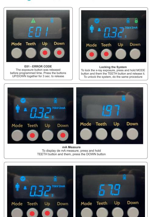
**kV Measure** To display de kV measure, press and hold TEETH button and them, press the UP button
