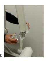
2. Apply the WD-40 as indicate on the pictures bellow (2.A, 2.B, 2.C). Clean the excess of the product and move the arm back and forward to see if the arm is smooth according your wish. In case it is put the white caps back and terminate the process, otherwise follow the next steps.
